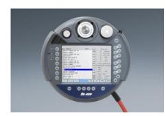
The control device, called Mobile Panel, features a colour graphics display and touch control.
